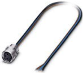
Sensor/actuator flush-type socket, 3-pos., M8, front/screw mounting, with M8 thread, with 1 m TPE litz wire, 3 x 0.25 mm 2
