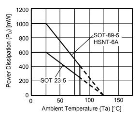
Figure 12 Power Dissipation of Package
