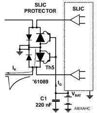
Figure 4. Negative Overvoltage Condition
