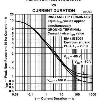
Figure 2. Non-repetitive Peak On-State Current against Duration (Gate Voltage Ranges are -20 V to -75 V for the '61089 and -20 V to -100 V for the '61089A)
