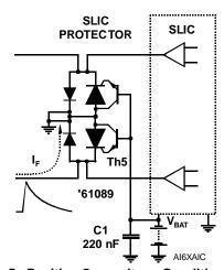
Figure 5. Positive Overvoltage Condition
