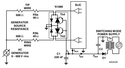
Figure 3. '61089 Buffered Gate Protector
