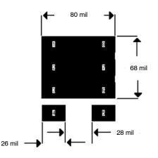
FIGURE 2. Footprint With Copper Spreading
