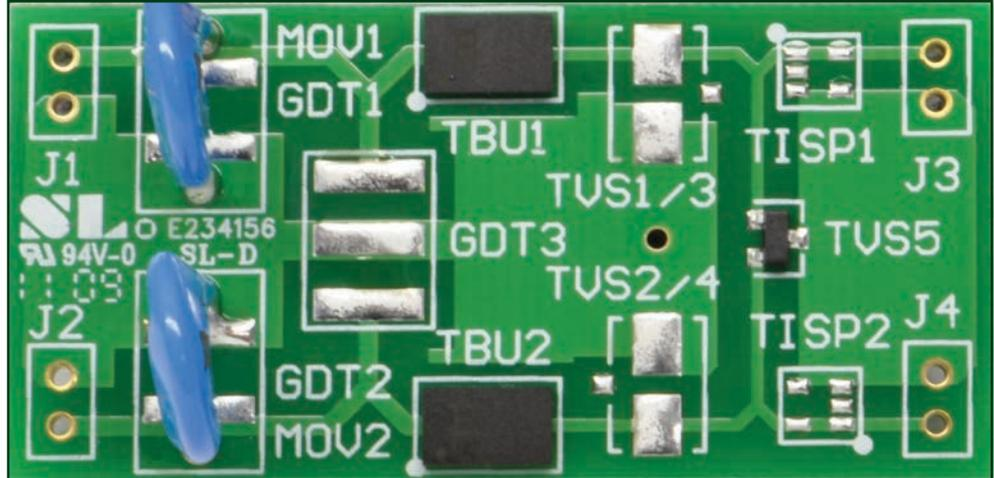
Figure 2 | RS-485 Evaluation Board 2 Top Side Layout\*
