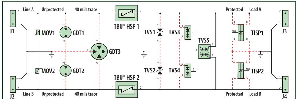
Figure 1 | RS-485 Evaluation Board 2 Schematic
