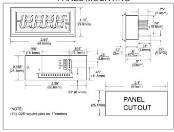
\*Note: If the input signal is not referenced to the power supply, pins 2 & 4 should be tied together for proper operation.
